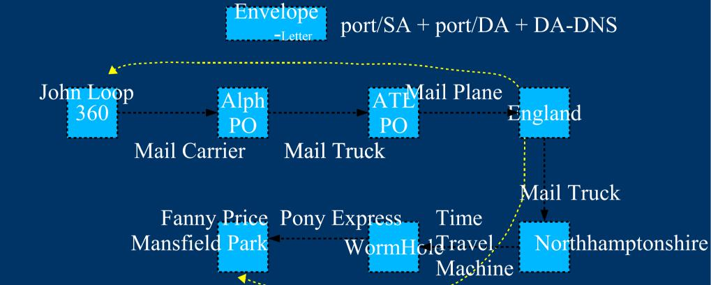
The Network Layer delivers the envelope (IP packet)
